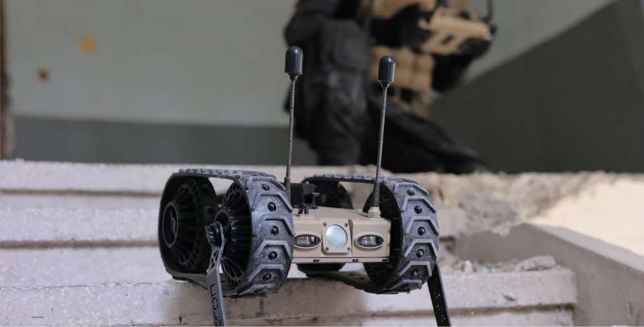
ESEBOT-50 offers high maneuverability with its tracked design and manipulator arms. It operates seamlessly with **IP65 protection** and **3 meters drop resistance**. Its self-righting and obstacle avoidance features maximize efficiency.
