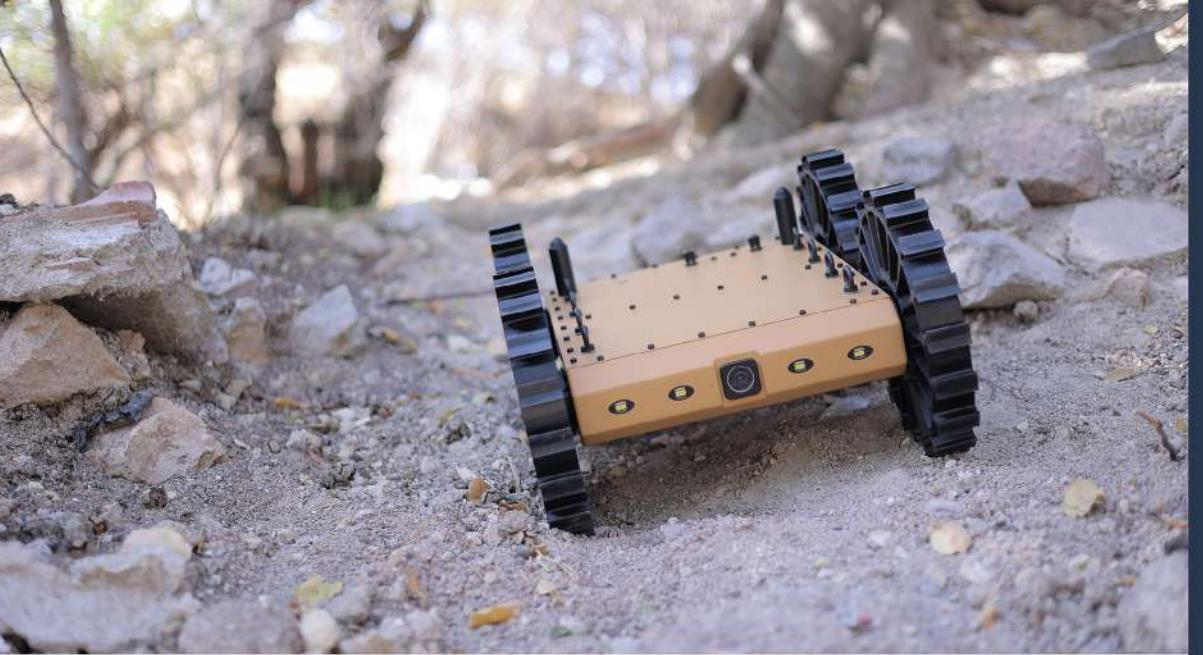
The integrated **HD camera** provides continuous surveillance in both indoor and outdoor environments, day and night. The **LED and IR illumination** systems allow for clear imaging even in low-light conditions.
